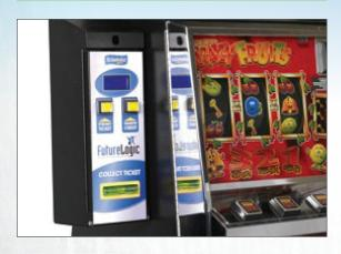
Small side box with credit transfer panel and ticket printer
