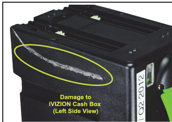
Figure 2: iVIZION Cash Box Exterior Surface Damage (Close Up)
