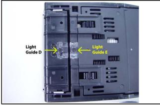
Figure 1: TR Light Guides D and E (iVIZION® Transport and Transport Cover)
